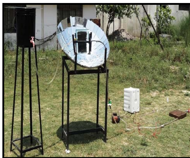
Fig 4.4 : Latent Heat Storage Solar Cooking Unit
