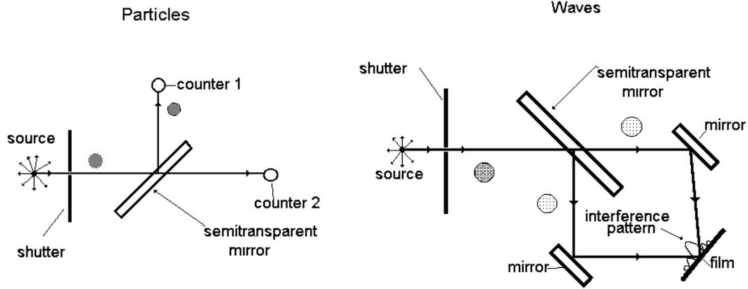
Figure 9: Experiments with individual photons on semitransparent mirror
