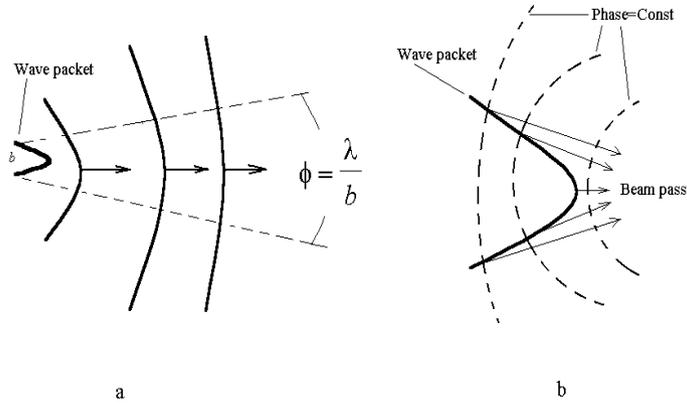
Figure 3 : Wave packet dispersion and refocusing
